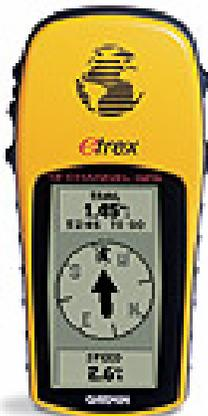
Most 12 parallel channel receivers are quick to lock onto satellites and are accurate, on average, to 15 meters. Certain atmospheric conditions, ravines, tall buildings, dense forests, and satellites on the horizon rather than right above you can affect the accuracy or cause signal loss. Newer and more expensive models have better accuracy; from 3 meters to the exact location.
